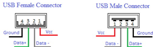
Figure 1: Structure of a USB port.
