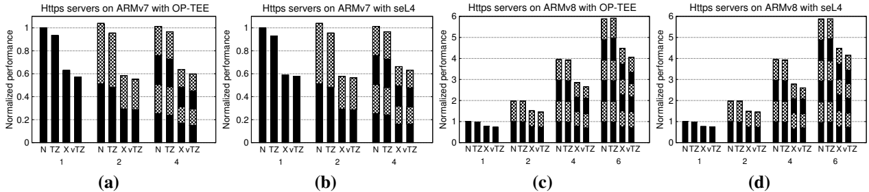
Figure 8: Multi-Guest (normalized throughput, higher is better), running 1, 2, 4, 6 GoHttp servers concurrently in native environment(N), native environment with TrustZone(TZ), original virtualization environment provided by Xen (X) and our system (vTZ). Figure (a) and (b) show the results on ARMv7 with OP-TEE and seL4 respectively. Figure (c) and (d) show results on ARMv8. The https server is GoHttp.
