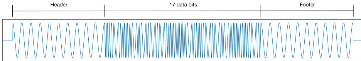
Figure 3: This 74ms modem transmission of a single frame demonstrates how data is modulated and wrapped in headers and footers for synchronization.
