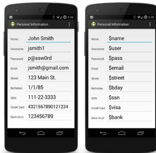
Fig. 2.1: On-screen sensitive data (left) and data protected by masking with cashtag aliases (right).
