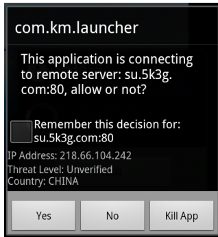
Figure 6: Enforcement of Network Policies: Access to an IP address with an unverified level of maliciousness
