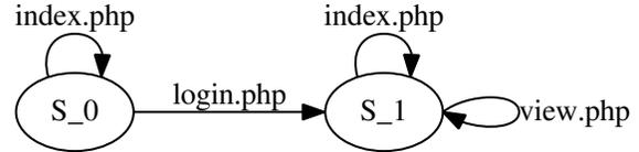
Figure 2: State machine of a simple web application.
