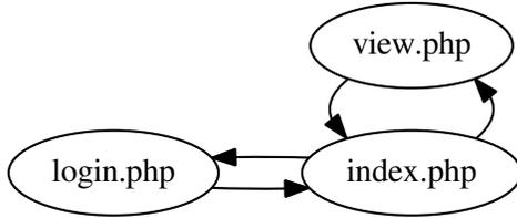
Figure 1: Navigation graph of a simple web application.
