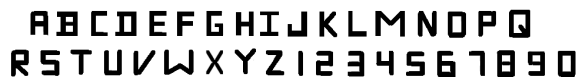
Figure 8: 14-segment LED font used for displaying letters and numbers in the study described in Section 4.3
