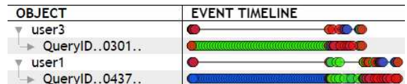
Figure 1: Stitch’s timeline graph. Each line represents an object with its IDs listed in the left panel. Users can drill down to objects at the next level by clicking on the object. Each circle in the right panel represents an individual event, and its color indicates the node where the corresponding log message was output. Only two out of many queries are shown.
