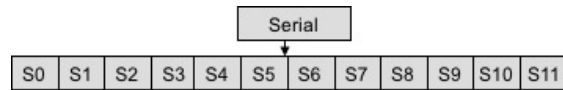
Figure 1: The structure of Classical Waffinity with the Serial affinity on top and the twelve Stripe affinities below.
