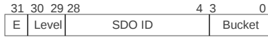
Figure 4: CleanOS Taint Tag Structure. We impose a structure on TaintDroid taints to support arbitrary numbers of taints.
