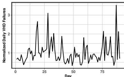
Figure 2: Daily VHD failures normalized by 3-month average. Every day had at least one failure. On the worst day there were 3.5x more failures than average.
