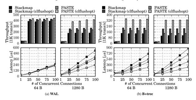
Figure 13: Throughput and mean latency with clflushopt.
