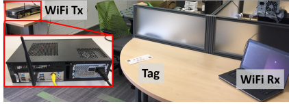
Figure 15: Experiment setup with commodity WiFi. the PCA to obtain the final tag response. This weakens more fading profiles that are likely to be uncorrelated, albeit at the cost of increasing detection latency.
