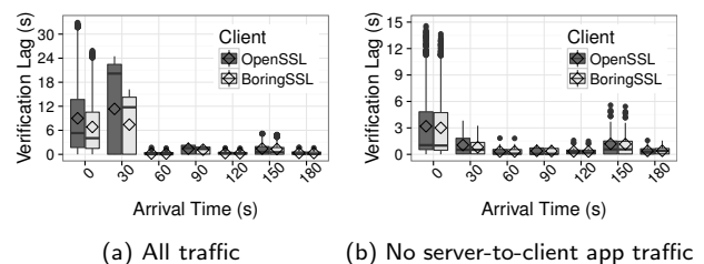
Figure 5: Verification lags for Gmail data set. Box plot at arrival time t includes \{lag(i) : t \leq arr(i) < t + 30s\} . Fig. 5a shows lags for all messages in all 21 TLS sessions. Fig. 5b shows lags if server-to-client application-data messages are dropped.
