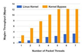
Figure 8: Throughput with and without kernel bypass.
