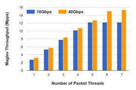
Figure 10: Throughput with different NIC speeds.
