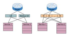
Figure 1: Hardware load balancer and Maglev.
