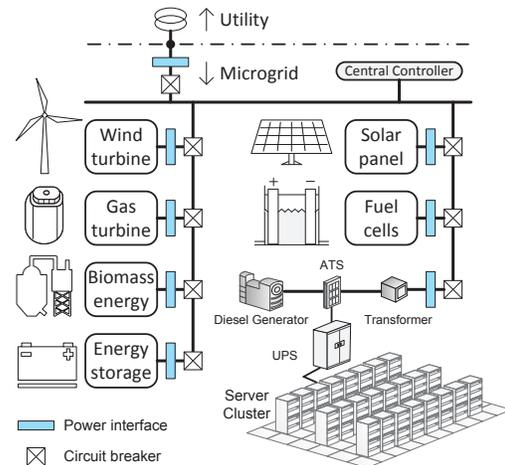
Figure 1: A datacenter powered by renewable power mix.
