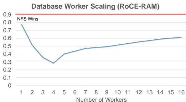
Figure 3: Performance of VHD configuration normalized by that of NFS in a test setup where data is stored in a RAM disk and accessed over a RoCE network.
