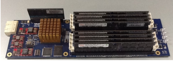
Figure 3: Our DRAM-based SSD Jetspeed™ hardware used to emulate PCM device connected with PCI Express Gen2 x4 channel
