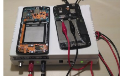
Figure 1: The test bench setup with Monsoon Power Monitor connected to Nexus 4 and Nexus 5.
