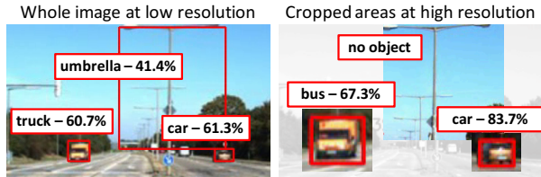
Figure 3: Inference results on low-resolution image (left) indicate where the protocol should “zoom-in” with high resolution (right) to improve the inference accuracy.
