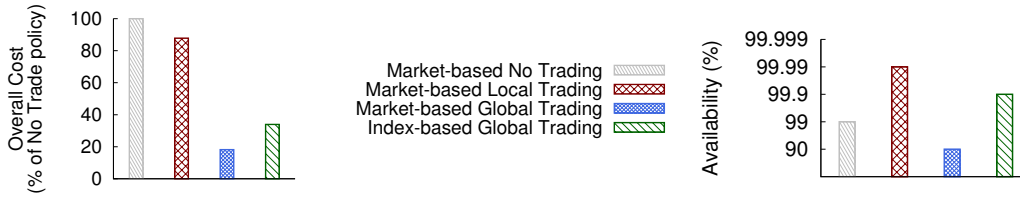
Figure 7: Comparison of cost and availability for our generic application using each of our four policy variants.
