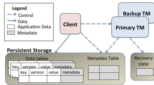
Figure 1: **Omid architecture.** Clients manipulate data that resides in data tables in the underlying data store (for example, HBase) and use the TM for conflict detection. Only the primary TM is active, and the backup is in hot standby mode. The TM maintains persistent metadata in the data store as well as separately managed recovery state (for example, using Zookeeper).
