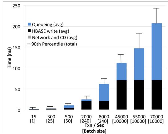
Figure 7: **Omid throughput vs. latency.** Client-perceived commit latency (average broken down and 90% of total); single region server; power-law transaction sizes with  $\alpha = 1.6$ ; batch sizes optimized for minimum latency (in square brackets below each bar).
