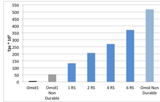
Figure 5: **Scalability of Omid’s CT updates with the number of HBase region servers, and comparison with Omid1.** Non-durable versions do not persist transactions and thus provide upper bounds on throughput under perfect storage scaling.
