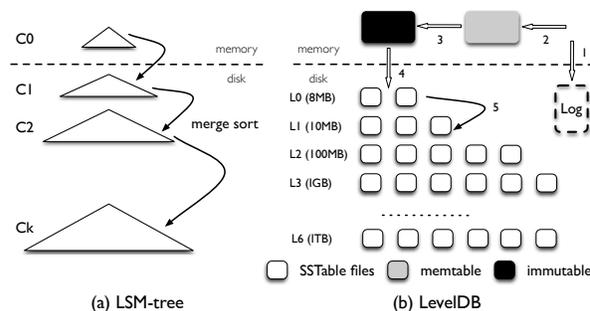
Figure 1: **LSM-tree and LevelDB Architecture.** This figure shows the standard LSM-tree and LevelDB architecture. For LevelDB, inserting a key-value pair goes through many steps: (1) the log file; (2) the memtable; (3) the immutable memtable; (4) a SSTable in L0; (5) compacted to further levels.
