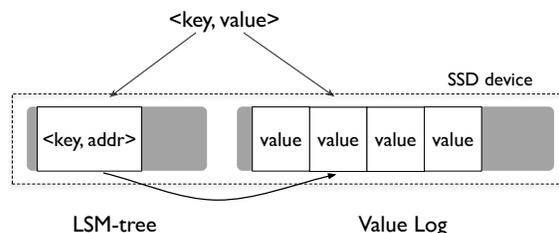
Figure 4: **WiscKey Data Layout on SSD.** This figure shows the data layout of WiscKey on a single SSD device. Keys and value’s locations are stored in LSM-tree while values are appended to a separate value log file.
