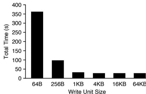
Figure 6: **Impact of Write Unit Size.** This figure shows the total time to write a 10-GB file to an ext4 file system on an SSD device, followed by a `fsync()` at the end. We vary the size of each `write()` system call.
