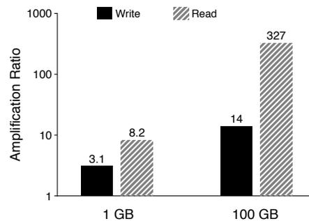
Figure 2: **Write and Read Amplification.** This figure shows the write amplification and read amplification of LevelDB for two different database sizes, 1 GB and 100 GB. Key size is 16 B and value size is 1 KB.
