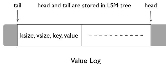
Figure 5: **WiscKey New Data Layout for Garbage Collection.** This figure shows the new data layout of WiscKey to support an efficient garbage collection. A head and tail pointer are maintained in memory and stored persistently in the LSM-tree. Only the garbage collection thread changes the tail, while all writes to the vLog are append to the head.
