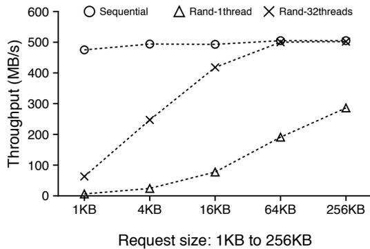
Figure 3: **Sequential and Random Reads on SSD.** This figure shows the sequential and random read performance for various request sizes on a modern SSD device. All requests are issued to a 100-GB file on ext4.
