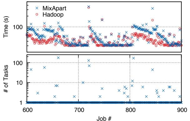
Figure 9: **Low Data Reuse Trace.** With many concurrent large I/O intensive tasks, the storage server gets bottlenecked causing subsequent tasks to be *backlogged* waiting for I/O requests to be scheduled.
