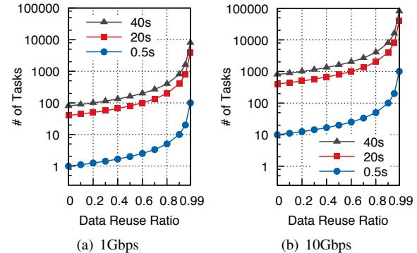
Figure 1: **Compute Cluster Size.** We show the number of parallel map tasks sustained by the cache + shared storage architecture for MapReduce analytics. Labels represent average map task durations – e.g., 0.5s for I/O intensive tasks. We plot values for cache-storage bandwidths of (a) 1Gbps, and (b) 10Gbps.
