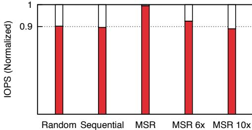
**Figure 10: Enterprise and Data Analytics Workloads on Shared Storage.** We show performance for enterprise workloads in I/O requests per second (IOPS) normalized to performance achieved with full storage access. Concurrently running enterprise and analytics workloads in MixApart causes little performance degradation in the normal case (MSR). With high I/O intensive enterprise workloads, quanta scheduling ensures performance isolation.
