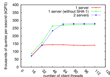
Figure 5: Performance evaluation of the KDS. A number of client threads requested leaf keys from one and two KDSes. It shows that one KDS sustains about 150 kQPS. The KHT settings were branch = 4 and depth = 11. After about 275 kQPS network became the bottleneck.
