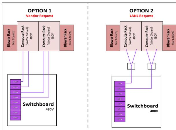
Figure 3 shows two facility designs for supplying power to the Trinity compute racks. Option 1 is the two 100-amp feed, vendor-proposed design. Option 2 is the modified J-Box design which uses a single 150 amp feed per rack.
