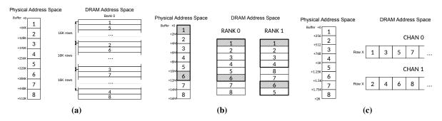
Figure 6: Examples of nonlinear DRAM address mappings taken from real systems [10, 49, 54].
