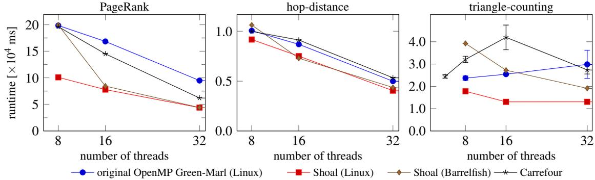
**Figure 4:** Scalability on 8x8 AMD Opteron. Workload: Twitter (LiveJournal for triangle-counting). For Shoal, we chose the best configuration each. We omit results for 64 threads: using SMT threads has similar performance to using only the 32 physical cores.
