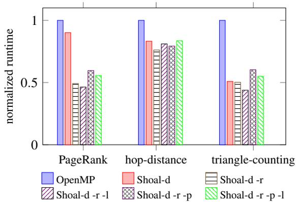
**Figure 6:** Comparison of various combinations of array implementations on 8x8 AMD Opteron: distribution (-d), replication (-r), partitioning (-p), large page (-l) (runtime normalized to stock-Green-Marl)
