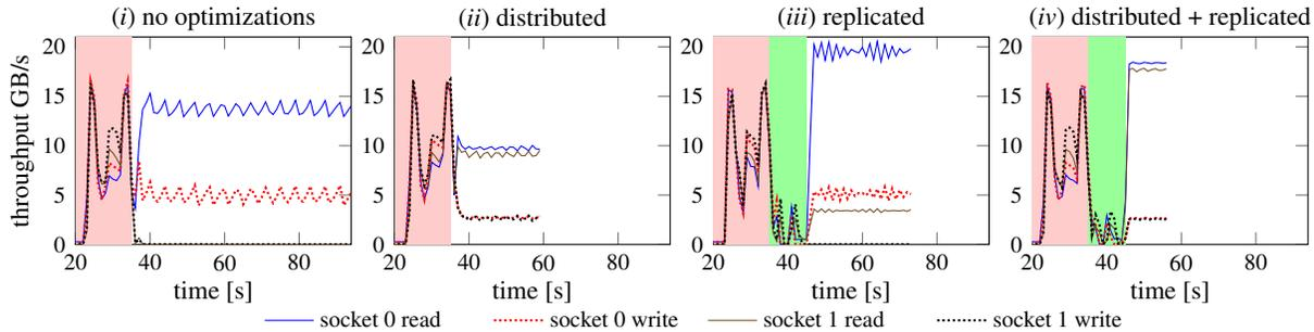
**Figure 7:** Memory throughput for sockets 0 and 1 on 4x8x2 Intel Xeon. In the first 35 seconds, the graph is loaded from disk. For replication, we show the replica initialization cost in green. Note: Sockets 2 and 3 are equal to socket 1 and left out for readability.
