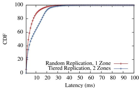
**Figure 8: Comparison of write latency between Tiered Replication across two availability zones and Random Replication on a single availability zone under YCSB benchmark.**
