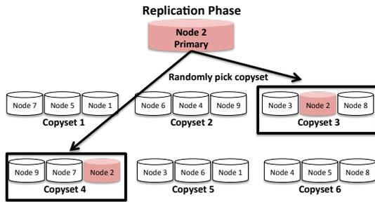
**Figure 5: Illustration of the Copyset Replication Replication phase.**
