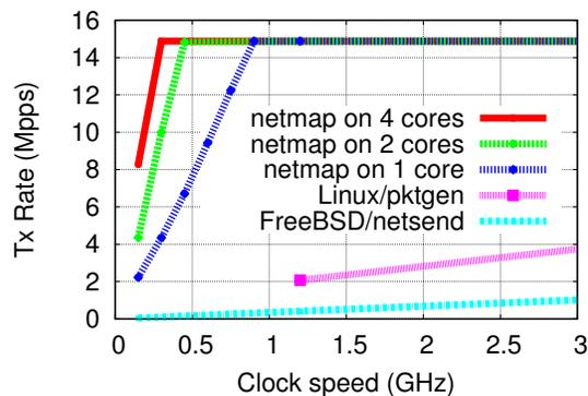
Figure 5: Netmap transmit performance with 64-byte packets, variable clock rates and number of cores, compared to *pktgen* (a specialised, in-kernel generator available on linux, peaking at about 4 Mpps) and a *net send* (FreeBSD userspace, peaking at 1.05 Mpps).
