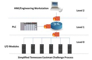
Figure 13: Segmented network architecture according to Purdue Reference Model
