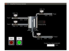
Figure 11: Operator Human Machine Interface (HMI)
