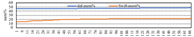
Figure 21: Memory utilization of Fixwindow tuned by Swift and with default configuration. The X axis represents samples.
