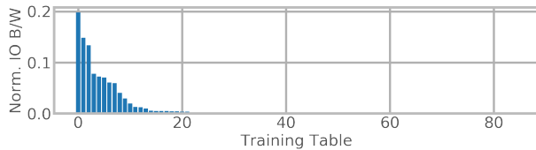
Figure 3: IO bandwidth demand across 85 tables over the course of one day. Training tables exhibit a power law in popularity.
