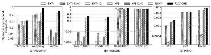
Figure 11: Performance comparisons of using real-world applications (a) Filebench, (b) RocksDB, and (c) MinIO.
