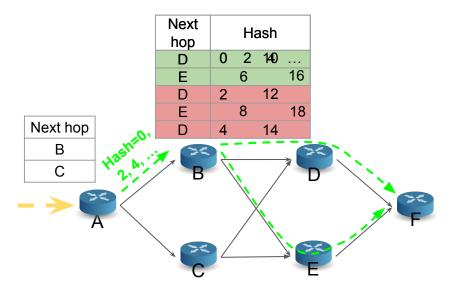
$A \rightarrow B \rightarrow E \rightarrow F$  is now used along with  $A \rightarrow B \rightarrow D \rightarrow F$ , with a traffic split of 2:3 (vs. intended 1:1).
