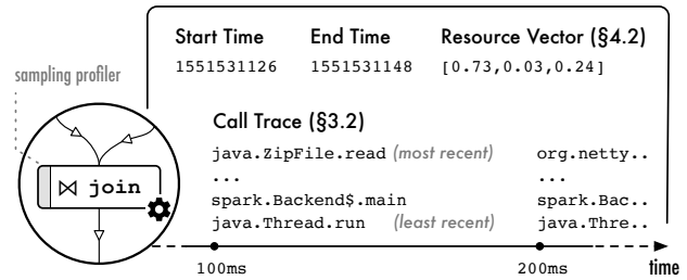
Figure 2: When a node (operation) is executing, attached is a sampling profiler for periodically sampling the call stacks. For each node, we build an execution profile to organize its resource-time information.
