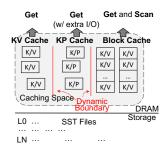
Figure 4: AC-Key Caching Components
