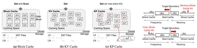
Figure 2: Three Types of Entries to Cache in LSM-KVS.
