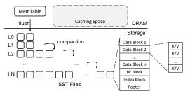
Figure 1: LSM-based Key-value Store (LSM-KVS).
