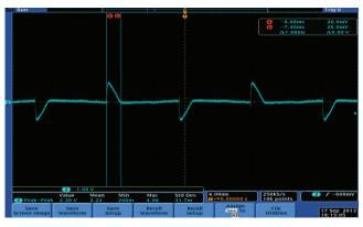
Figure 11: Plot of voltage across the terminals of the CFL with dimmer level set to 8.
