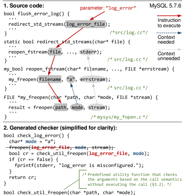
Figure 4: Illustration of PCHECK’s checker generation (using a real-world LC error example [26]). PCHECK replaces the original call ( freopen ) with check utilities based on access and stat to prevent side effects (§3.2). To execute the instructions, the necessary execution context needs to be produced. Note that we illustrate the checker using C code for clarity; the actual code is in LLVM IR or Soot Jimple.
