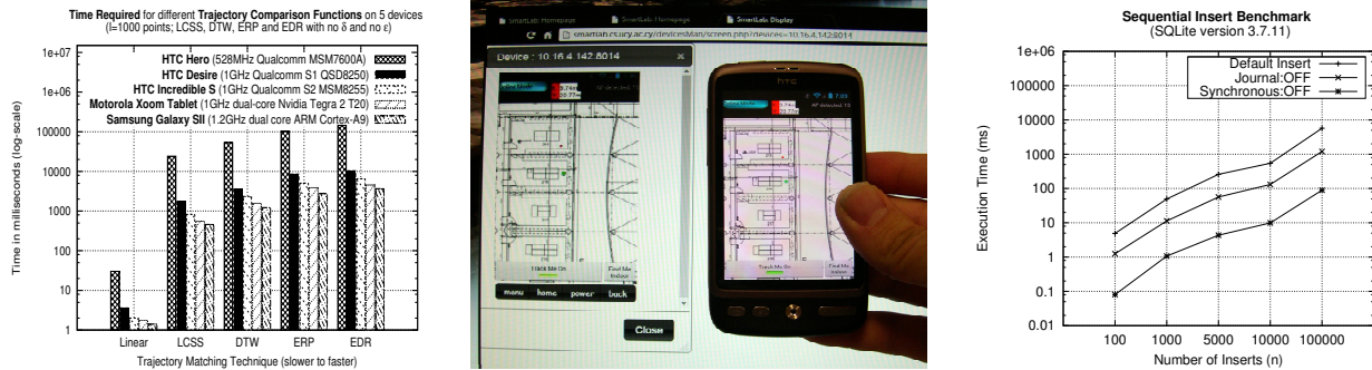
Figure 14: Research with SmartLab. (Left) Testing trajectory comparison algorithms on a diverse set of smartphones in SmartTrace [38]; (Center) Testing indoor localization using ARD-WiFi mode in Airplace [24]; (Right) Testing various SQLite tuning parameters in the context of an advanced databases course.
