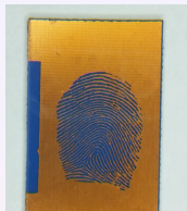
(c) Etched PCB negative
