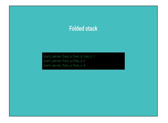
Folded stack is one example of an intermediate representation of trace data - puts stack traces on a single line, with functions separated by semicolons, followed by a space and then a unit - e.g a count.
