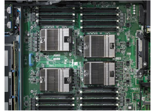
4-ways AMD multi-sockets (DELL PowerEdge R815)
