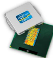
Sandy Bridge CPU 6 cores, 2.2 GHz
