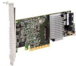
Intel RS3 RAID 1GB flash-backed cache 25 us / 1KB write
