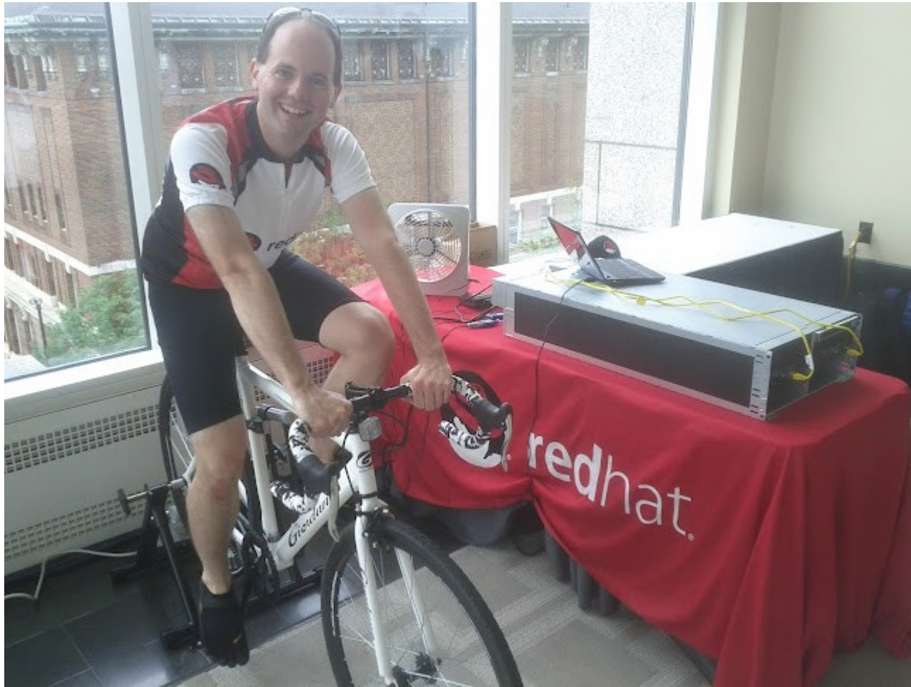
World's first bicycle-powered ARM Server (HP Redstone/Calxeda)
