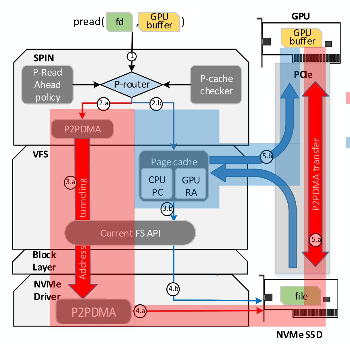
P2P: Address tunneling mechanism P\$: Memcpy from P\$ to **GPU** mapped memory
