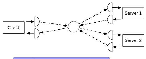
Separate input, processing and output tasks enable parallelism
