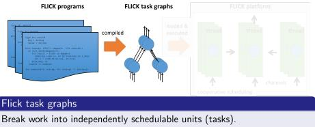
Join tasks by channels into task graphs.
