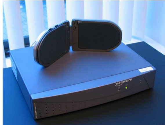
Figure 6: The Ethernet Speaker is based on the Neoware EON 4000.
