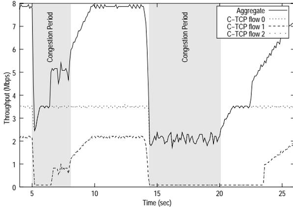
Figure 10: A constant bandwidth C-TCP flow with two C-TCP flows sharing remaining bandwidth.
