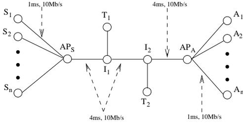
Figure 6: Simulation testbed in ns2.
